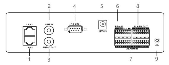
Figure 1-10 iDS-6700NXI-I/16S(B) Series Rear Panel
