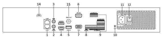
Figure 1-8 iDS-7700NXI-I4/16S(B) Series Rear Panel
