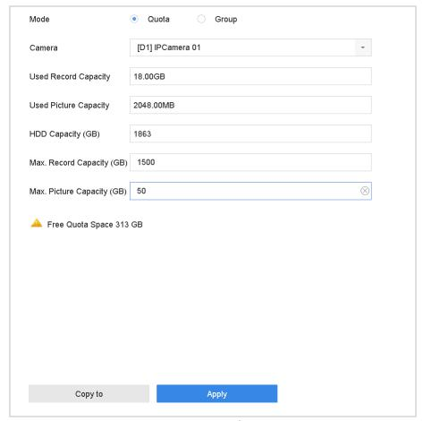
Figure 7-7 Storage Mode-HDD Quota
