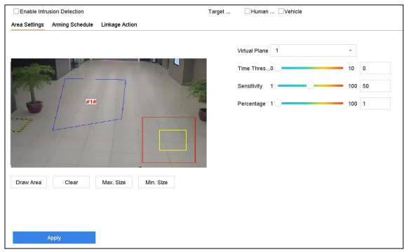
Figure 12-4 Intrusion Detection
