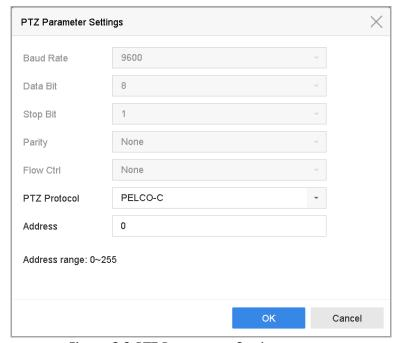
Figure 6-2 PTZ Parameters Settings
