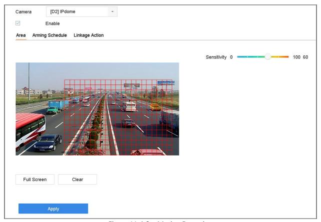
Figure 11-4 Set Motion Detection
