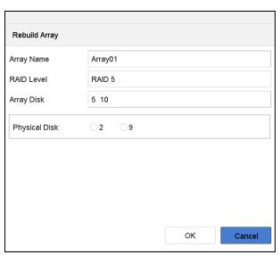
Figure 8-7 Rebuild Array
