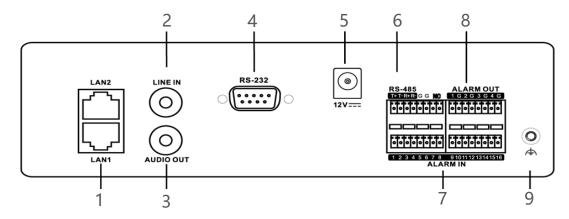
Figure 1-13 iDS-6700NXI-I/16S(B) Series Rear Panel
