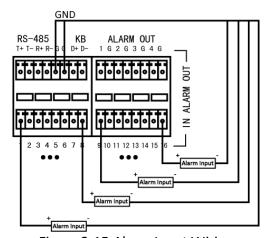
Figure 2-15 Alarm Input Wiring
