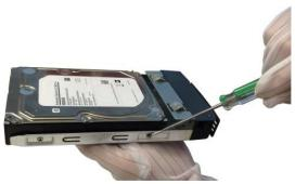
Figure 2-4 Fix the Hard Disk
