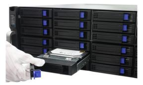
Figure 2-5 Push the Dummy HDD into the Slot
