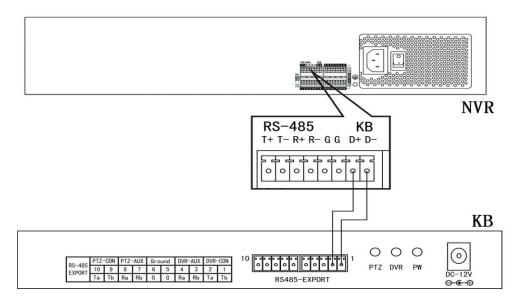
Figure 2-17 Controller Connection
