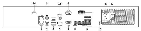
Figure 1-11 iDS-7700NXI-I4/16S(B) Series Rear Panel
