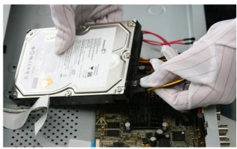
Figure 2-10 Connect Power Cable
