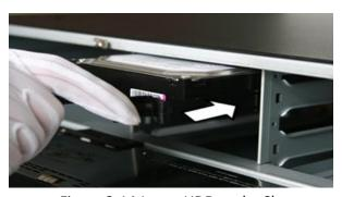
Figure 2-14 Insert HDD to the Slot
