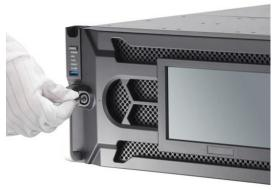
Figure 2-1 Unlock the Panel
