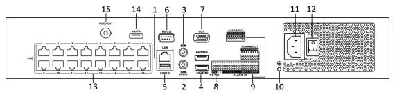
Figure 1-12 iDS-7700NXI-I4/16P/16S(B) Series Rear Panel
