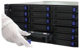
Figure 2-3 Pull out Dummy HDD
