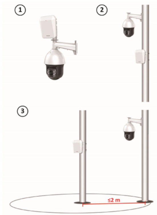
Figure 9-18 Scenario of One-Point Calibration
