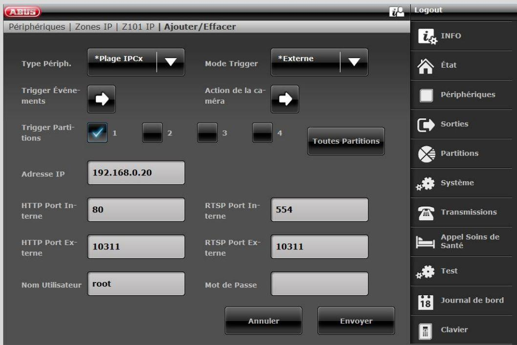
The screenshot shows the 'Ajouter/Effacer' (Add/Delete) configuration screen for an IP camera in the ABUS system. The interface is dark-themed and includes a sidebar menu on the right with options like 'INFO', 'État', 'Périphériques', 'Sorties', 'Partitions', 'Système', 'Transmissions', 'Appel Soins de Santé', 'Test', 'Journal de bord', and 'Clavier'. The main configuration area contains the following fields and controls:
