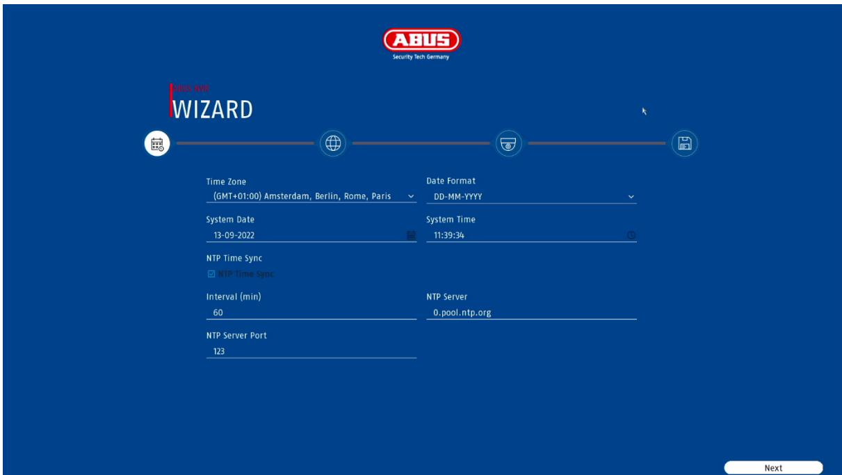
The setup wizard guides you through the necessary basic settings of the system. After that, the recorder is basically set up for recording and monitoring.
